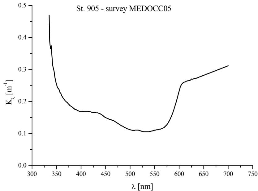
**Figure 20 Spectral attenuation profile ( $\text{m}^{-1}$ ) determined for the water mass between 2.5-18.5 m at St. 905.**
