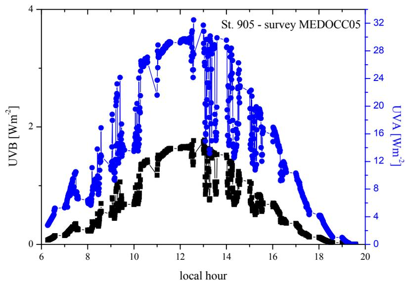
**Figure 22** Above surface solar irradiance in the UVB and UVA bands ( $\text{Wm}^{-2}$ ). The X-axis represents the local hour. Measured performed using a Skye radiometer positioned on the bow of the vessel.
