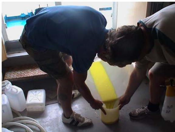
transferred in open polyethylene containers, and vigorously stirred; a known amount of  $^{134}\text{Cs}$  was added as yield tracer; the pH was adjusted to 1.5, adding HCl to 37%. Then, 15 g of ammonium molybdophosphate (AMP) were suspended in 50 ml of distilled water and the suspension was added to the sample. Stirring was continued for 3-4 hours. The AMP was left to settle down for 6-8 hours.
