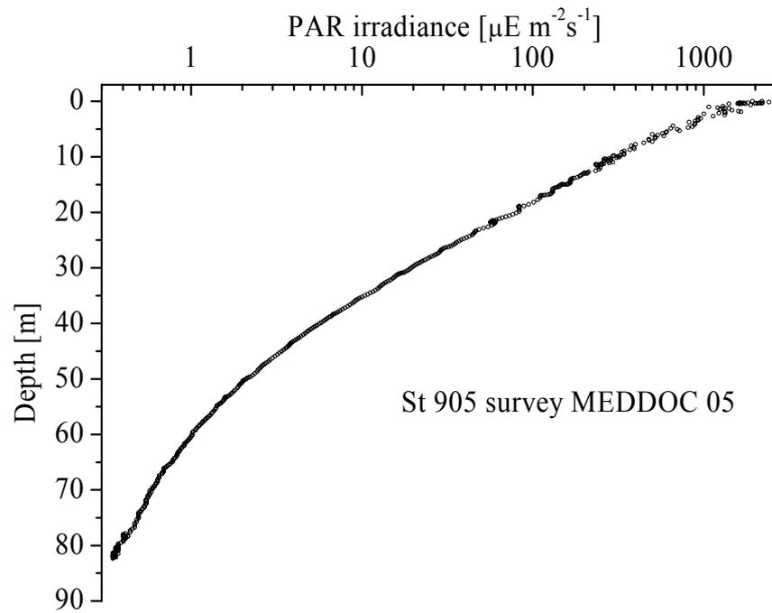
Figure 24 PAR irradiance profile ( $\mu\text{E m}^{-2} \text{s}^{-1}$ ) vs. depth (m).
