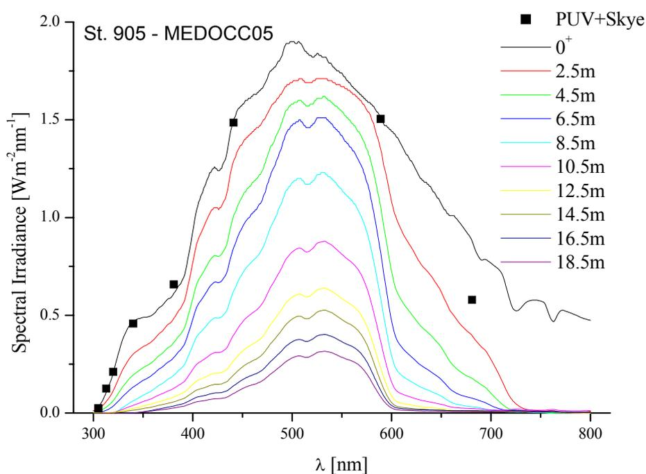
**Figure 19 Spectral irradiance ( $\text{Wm}^{-2}\text{nm}^{-1}$ ) as a function of wavelength (nm) in the first 18.5 m of the water column (St. 905). The black squares represent PUV 541 and Skye measurements at the water surface ( $0^+$ ).**
