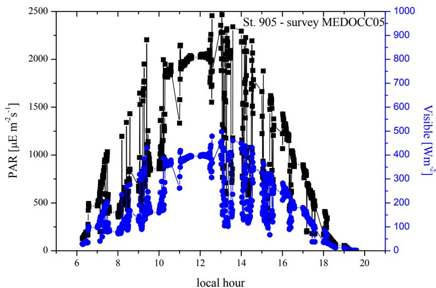
**Figure 23** In-air PAR irradiance ( $\mu\text{Em}^{-2}\text{s}^{-1}$ ) and visible irradiance ( $\text{Wm}^{-2}$ ). The X-axis represents the local hour. Measured performed using a Skye radiometer positioned on the bow of the vessel.
