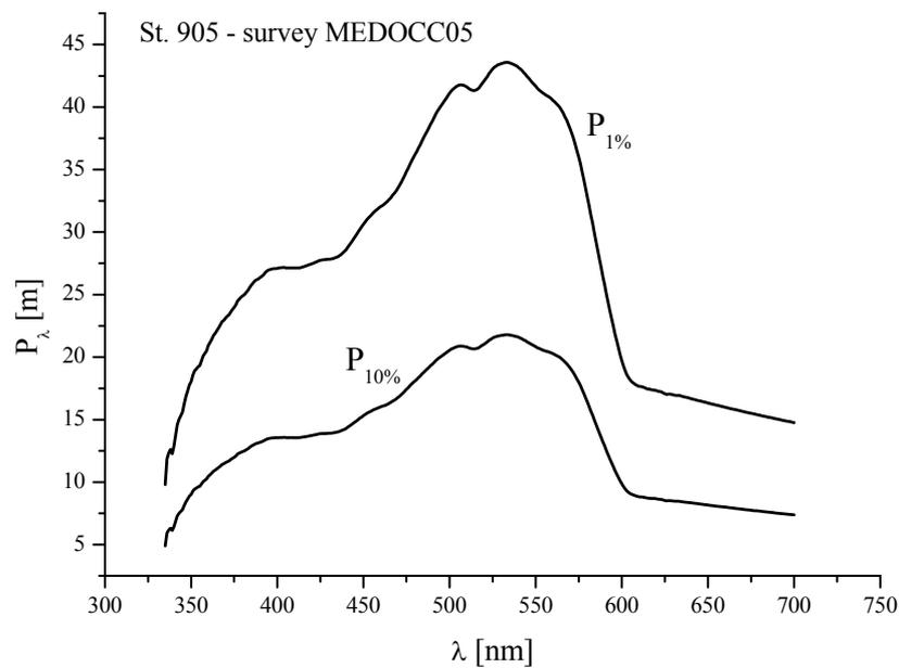
**Figure 21 Penetration depths of 1% and 10% of the sub-surface irradiance values ( $P_{1\%}$  and  $P_{10\%}$ ) by wavelength.**
