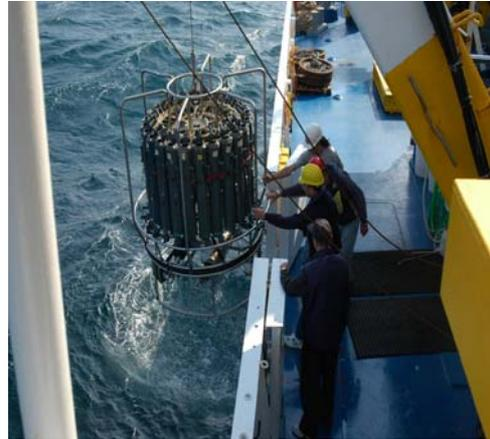
S/m. In addition, salinities of water samples were analysed on board using a Guildline Autosal salinometer. Dissolved oxygen was measured with a SBE-13 sensor (resolution 4.3  $\mu$ M), and data were checked against Winkler titration. The vertical profiles of all parameters were obtained by sampling the signals at 24 Hz, with the CTD/rosette going down at a speed of 1 m/s. The data were processed on board, and the coarse errors were corrected.
